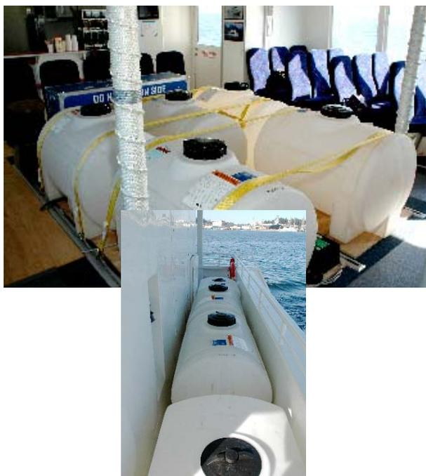
*Water tanks are used for extra ballast. This technique has been used to account for the weight of up to 149 passengers.*
