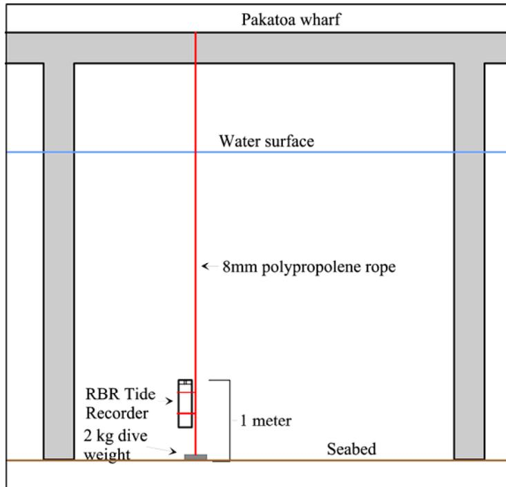
**Figure 3** Mooring system for the RBR Tide gauge deployed from the Pakatoa wharf
