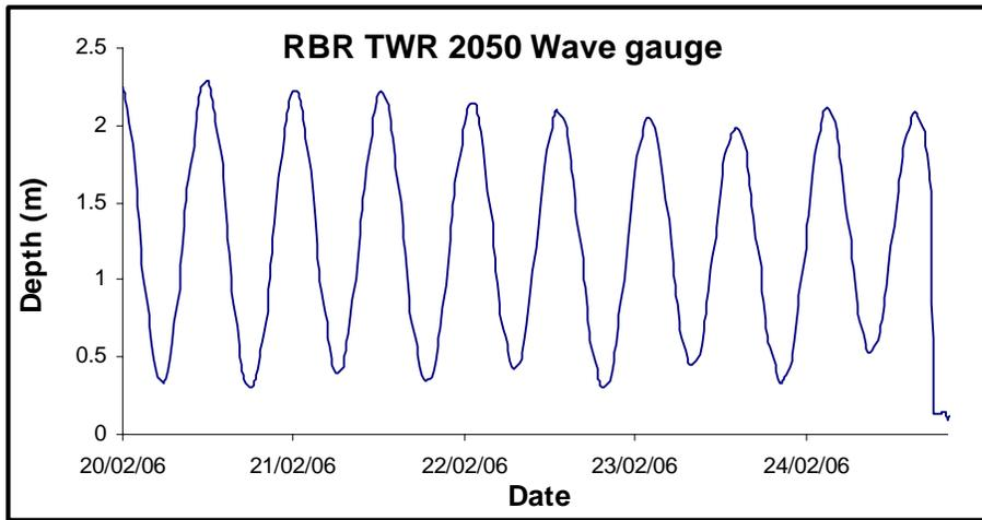
**Figure 4** Water levels recorded on the 20 m mooring
