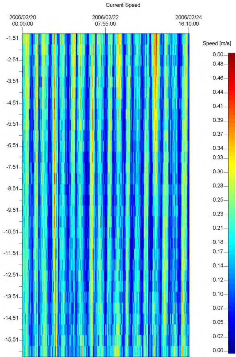
**Figure 11** Current speed profile measured on the 30 m mooring over the experimental period.
