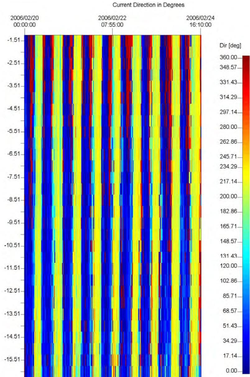
**Figure 12**      **Current direction profile measured on the 30 m mooring over the experimental period.**
