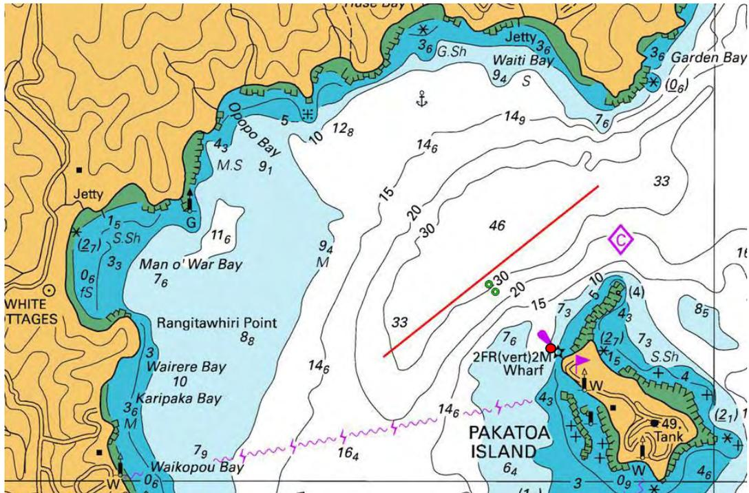
**Figure 1** North end of Waiheke Channel (Pakatoa Channel) showing the area of the wake tests with “Ten Sixty”. The red line shows vessel track; green circles show the locations of the 2 wave gauge moorings and red circle shows location of the tide gauge.
