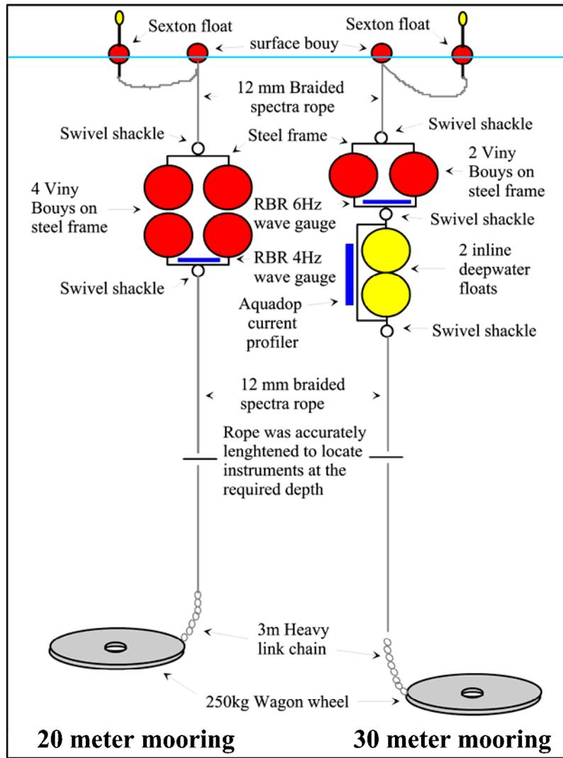
Figure 2 Mooring schematic.
