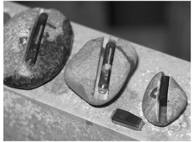
Fig. 4. RFID transponders – 32, 23, and 12 mm, respectively placed in tracer particles.
