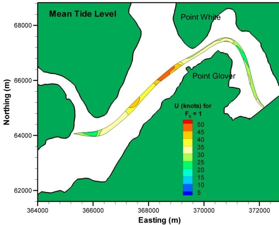
**Fig. 5. Critical speeds in Rich Passage – Sinclair Inlet along the Seattle – Bremerton passenger-only ferry route at mean tide level.**
