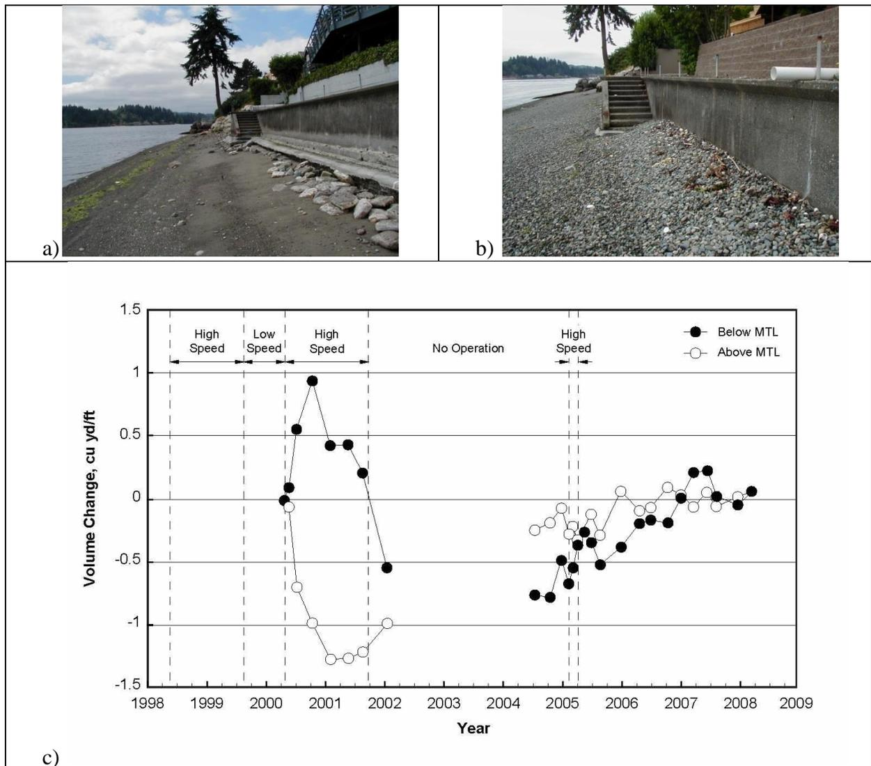
**Fig. 7. Photographs of a section of beach on Point White, Bainbridge Island in Rich Passage in July 2000 following 2 months of POFF operation (a) and in August 2004 following beach recovery (b).**
