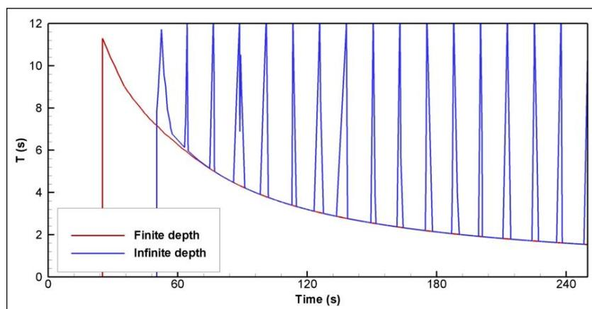
Fig. 2. Comparison of wake period at 300 m from the sailing line for finite and infinite depth cases
