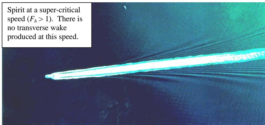
**Fig. 4. Photograph of Spirit at a super-critical speed. Note only diverging wakes are present.**
