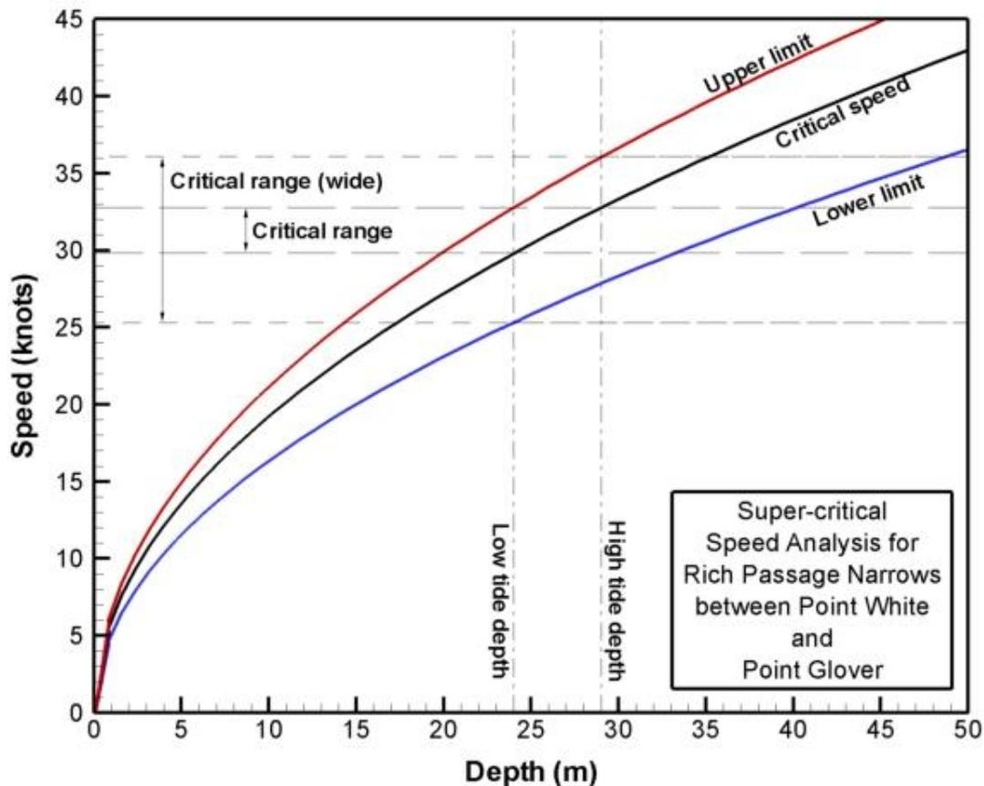
Fig. 6 Critical speeds analysis for Rich Passage Narrows between Point White and Point Glover
