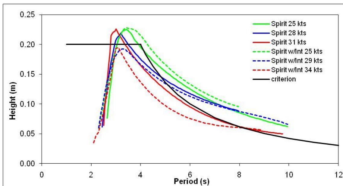
Fig. 8. Comparison of measured height spectrum for M/V Spirit operating at speeds between 25 and 35 knots, compared M/V Spirit with Interceptors and the new wake criterion.
