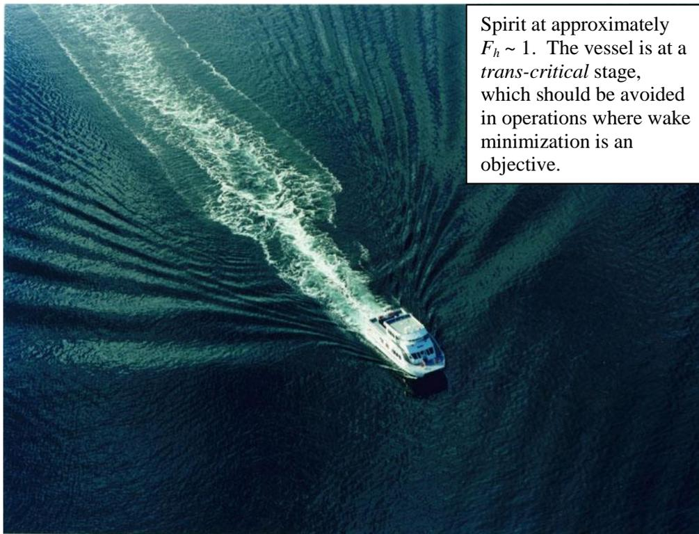
**Fig. 3. Photograph of Spirit slowing down and passing through the trans-critical speed. Note the large, long waves building alongside the vessel.**
