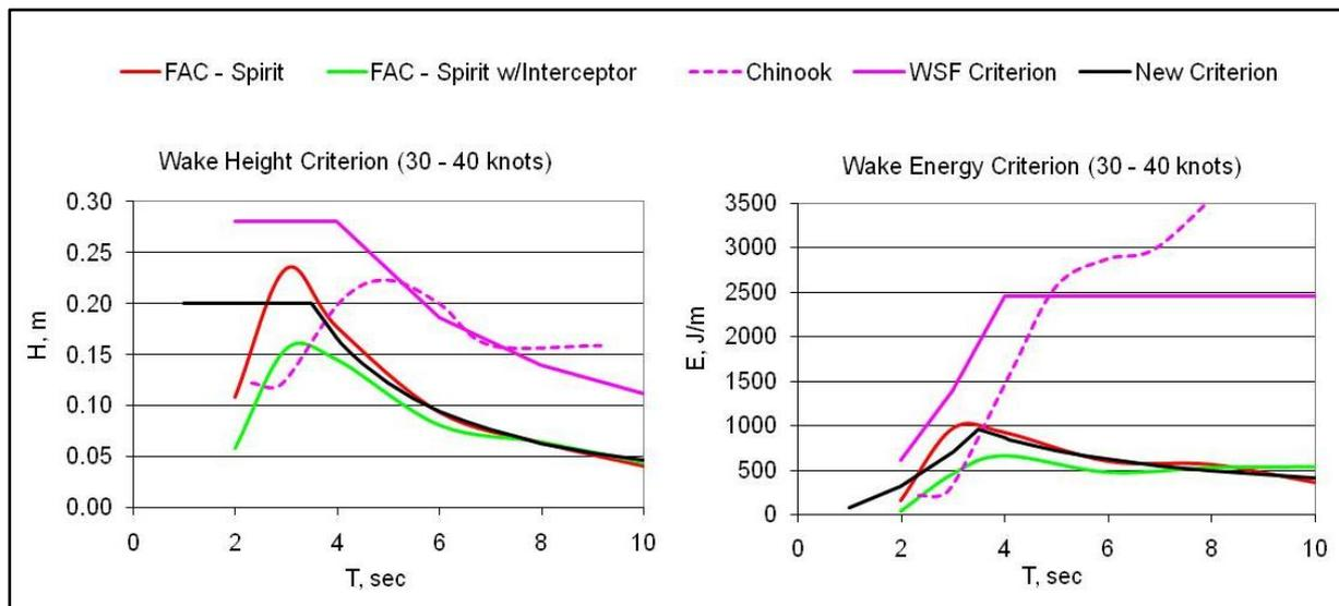
**Fig. 9. Comparison of measured height and calculated energy spectrum for foil-assisted catamarans and POFF operating at 30 to 40 knots, compared to previous wake height criterion set by WSF and new wake performance criterion.**
