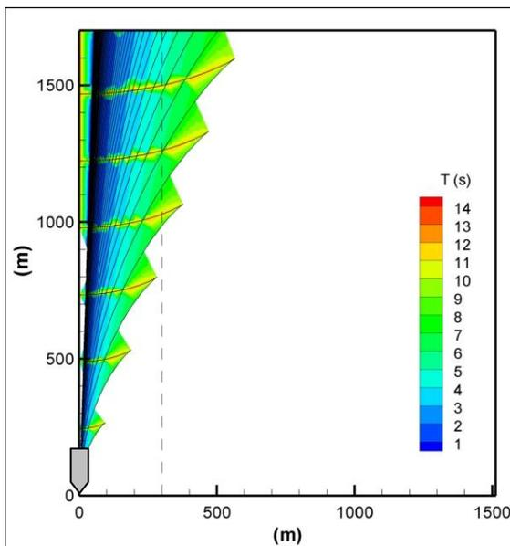
Fig. 1a. Wake period for 38 knot vessel in infinite depth water
