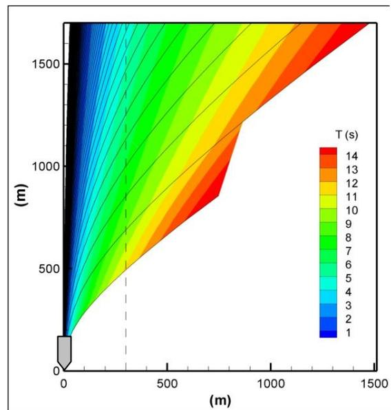
Fig. 1b. Wake period for 38 knot vessel in finite depth water
