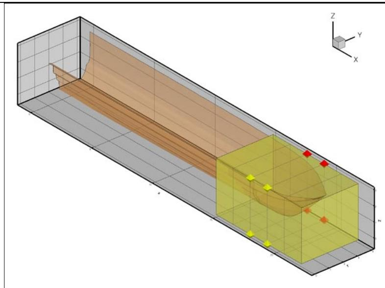
Fig 3: Perspective view of the FFD parameterization. Control points are represented by symbols.
