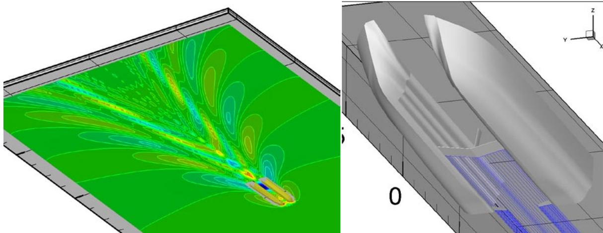
Fig 2: Predicted wave pattern for  $Fr = 0.6$  (left) and straight trailing vortices leaving the foils (left).
