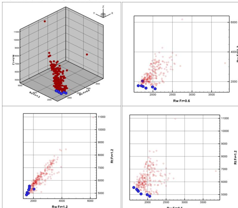
Figure 10: Different views of the resulting Pareto front: from top to bottom, left to right, a perspective view of the Pareto front, and three different views of the Pareto solutions projected onto the planes at constant F1, F2 and F3 values, respectively.
