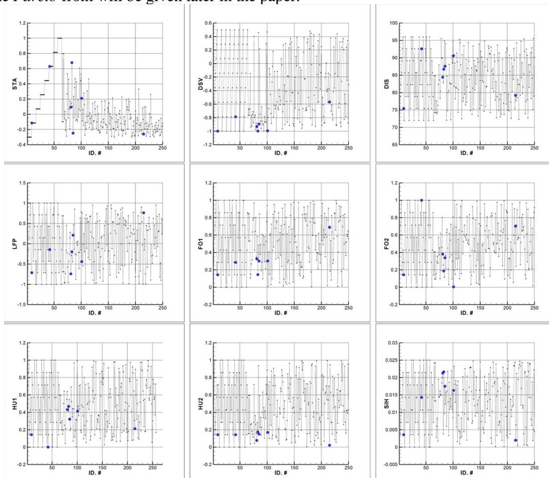
Figure 8: Values of the design variables as a function of the iteration of the optimization algorithm. The blue dots represents the values corresponding to designs that were found to be on the *Pareto* front.
