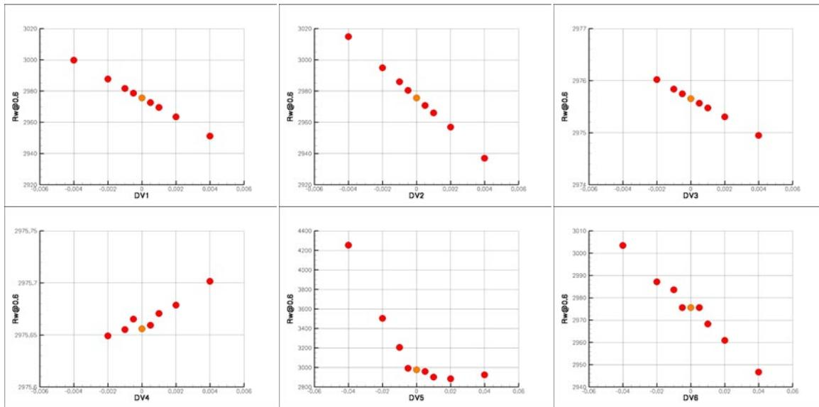
Figure 4: Sensitivity study: trend of the 6 design variables (in abscissa) with respect to the first objective function (wave resistance at  $Fr=0.6$ ).
