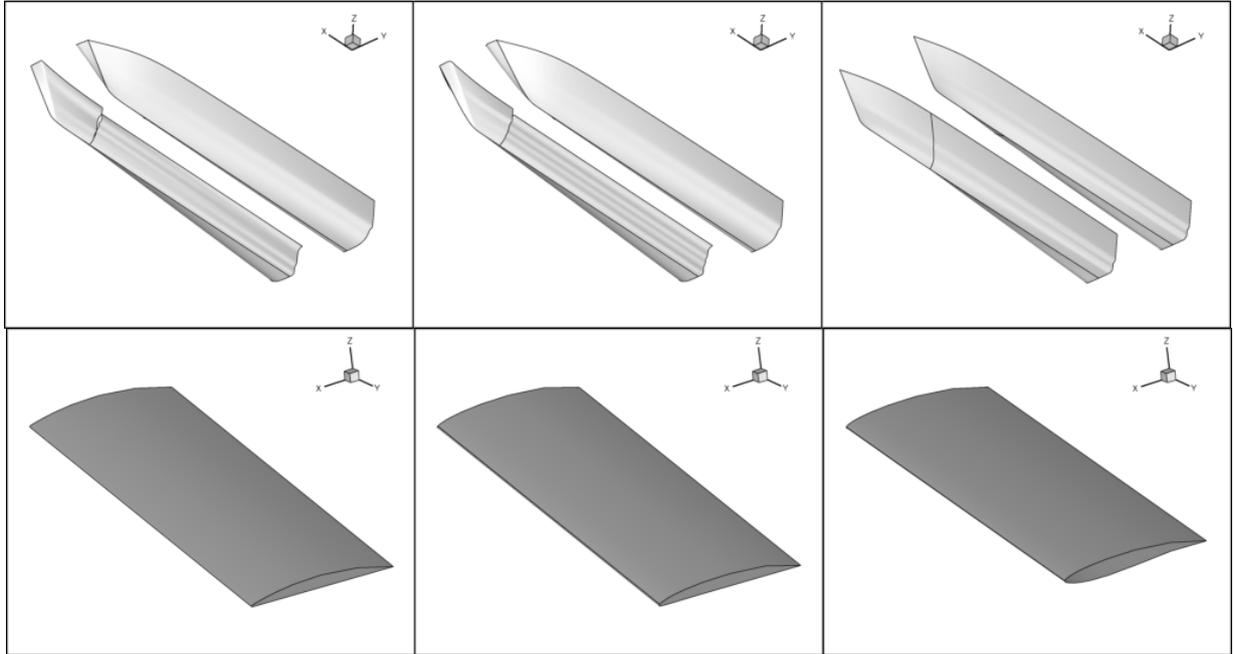
Figure 7: Perspective views of the three initial shapes of the demihulls and of the central foils adopted as a starting point for the design optimization of RV2. A couple of stern flaps as for SPIRIT are also adopted, being the same for all the given configurations (their shape is not reported here).
