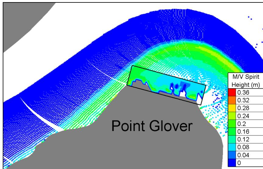
**Figure 11:** Instantaneous wake height pattern on the Point Glover shore from a Seattle-bound *M/V Spirit* at 37 knots (see text for description)
