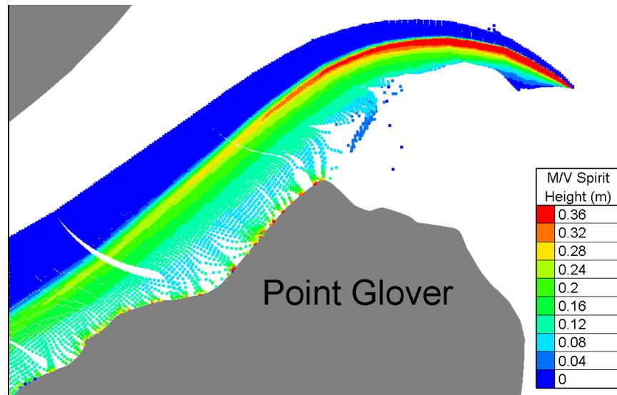
**Figure 10:** Example *LSV* solution for instantaneous wake height on the Point Glover shore from a Seattle-bound *M/V Spirit* at 37 knots. (Note: only starboard wake shown)
