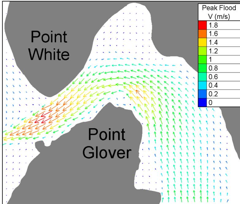
Figure 4: Tidal current pattern for Peak Flood case
