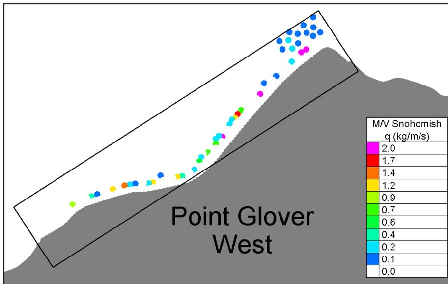
**Figure 20: Maximum potential sediment transport rate for *M/V Snohomish* Bremerton-bound at 37 knots and peak ebb at Point Glover West**
