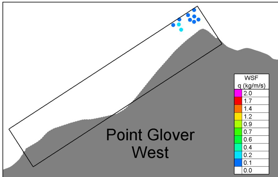
**Figure 22:** Maximum potential sediment transport rate for a WSF car ferry Bremerton-bound at 17 knots and peak ebb at Point Glover West
