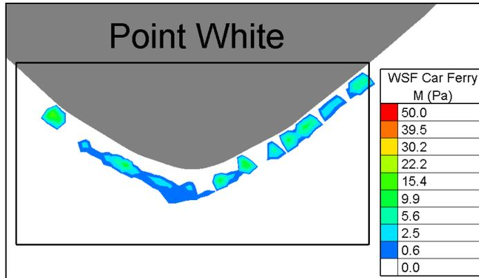
**Figure 12:** Maximum excess shear stress on the Point White shore from a Seattle-bound WSF car ferry at 17 knots and mid-tide
