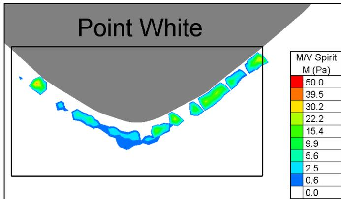
**Figure 13:** Maximum excess shear stress on the Point White shore from a Seattle-bound *M/V Spirit* at 37 knots and mid-tide
