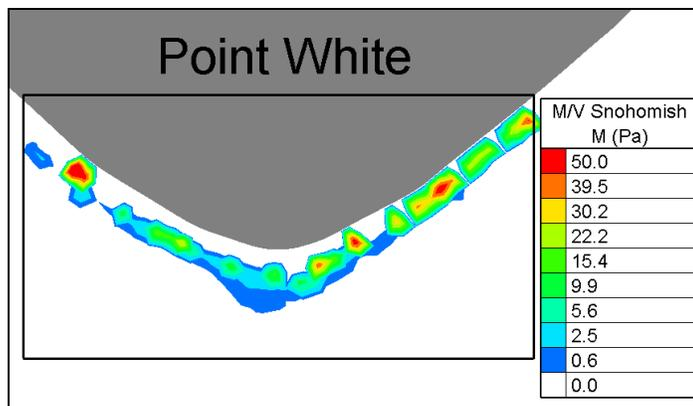
**Figure 14:** Maximum excess shear stress on the Point White shore from a Seattle-bound *M/V Snohomish* at 37 knots and mid-tide
