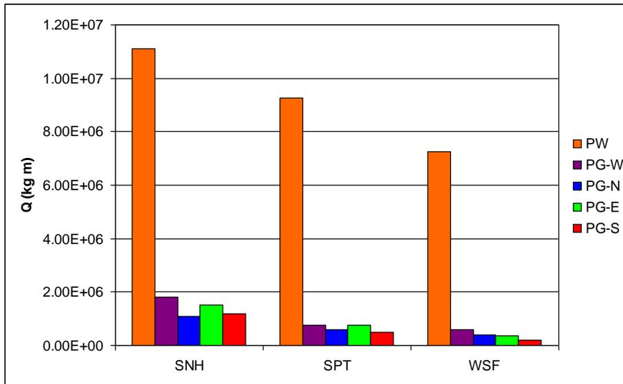
**Figure 25:** Sediment transport indicator for each vessel by site
