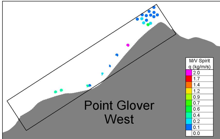
**Figure 21:**Maximum potential sediment transport rate for *M/V Spirit* Bremerton-bound at 37 knots and peak ebb at Point Glover West
